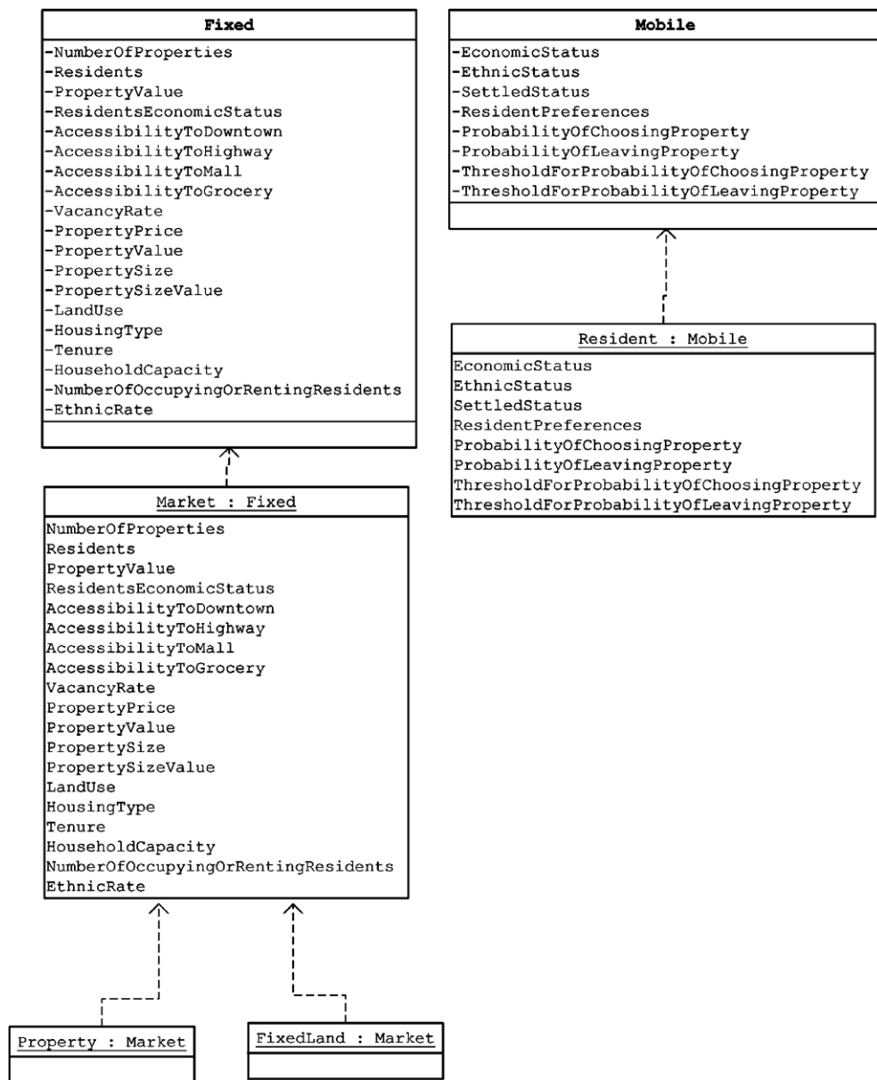
Fig. 1. Structural hierarchy of modeled automata entities.
